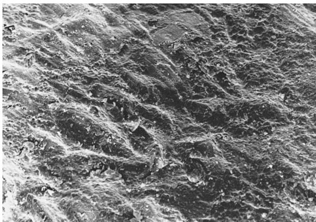
FIG. 2 Sandblasting for 5 seconds.
