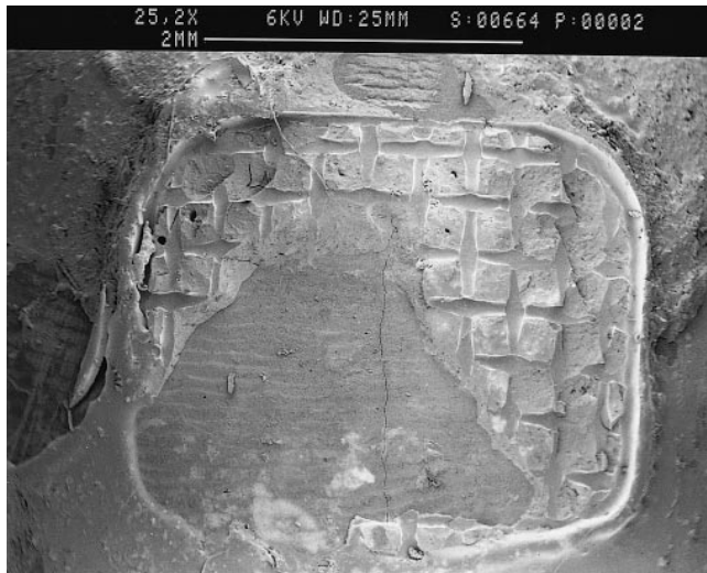
FIG. 5 Mixed mode of bond failure for etched specimen.
